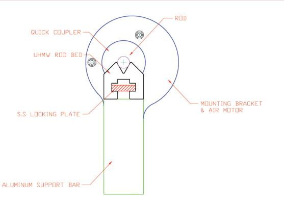
The ROD HOLDER can support coating rods down to 1/4" diameter.
